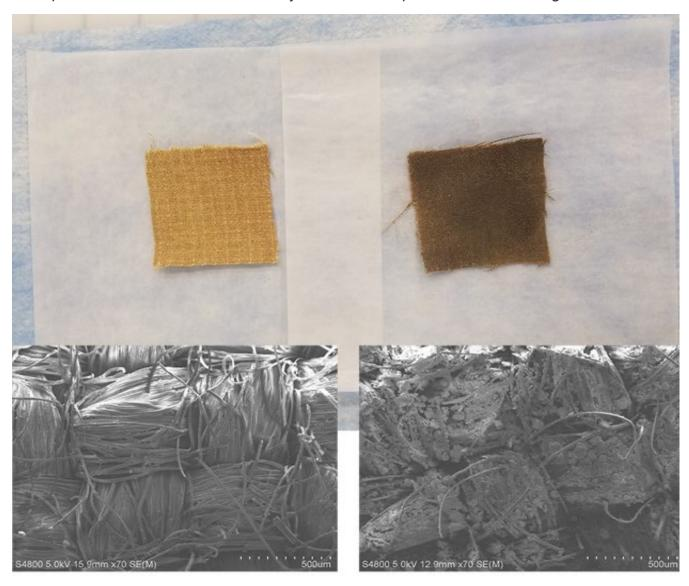
The images above are clean and soiled turn out coat fabric swatches side-by-side with electron microscope photographs showing dirt particles embedded in the soiled swatch under extreme magnification. (*Photo courtesy of the NIOSH National Personal Protective Technology Laboratory and Health Effects Laboratory Division.*)
