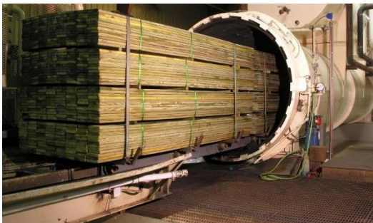
Pressure treated lumber being manufactured
