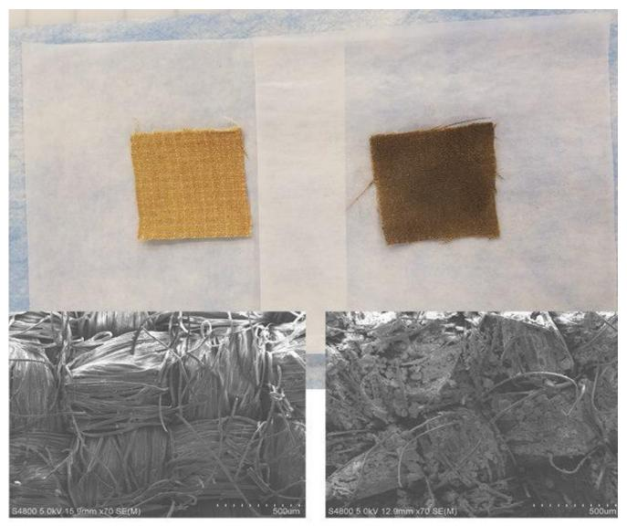
The images above are clean and soiled turn out coat fabric swatches side-by-side with electron microscope photographs showing dirt particles embedded in the soiled swatch under extreme magnification. (*Photo courtesy of the NIOSH National Personal Protective Technology Laboratory and Health Effects Laboratory Division.*)
